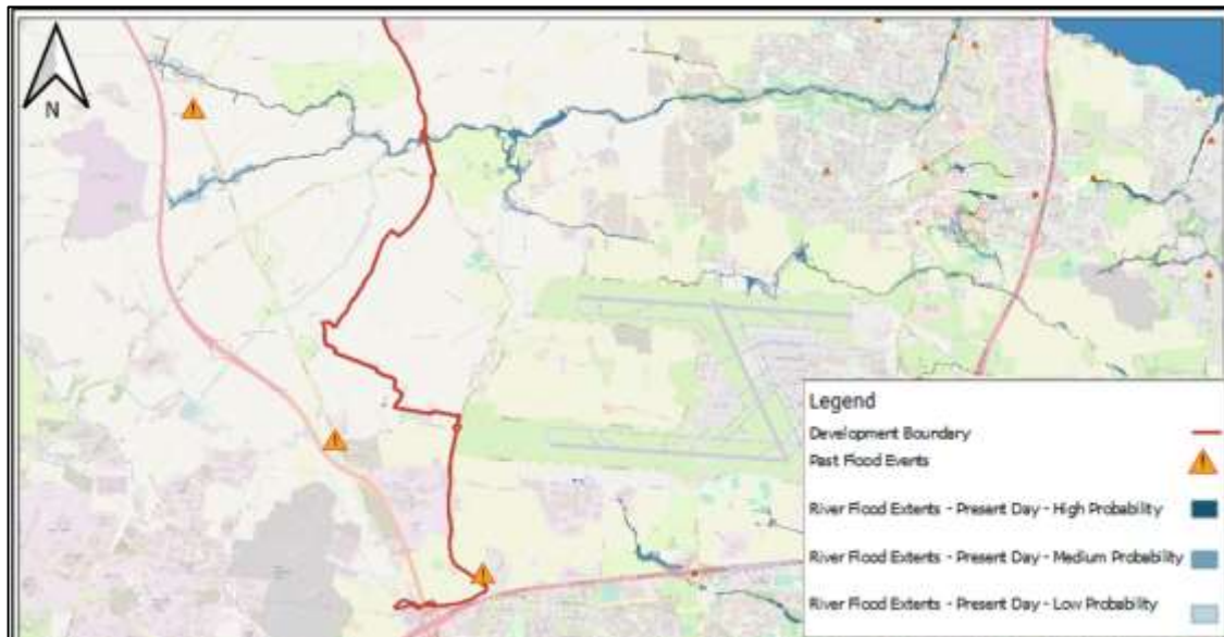
Figure 4-3: Flood Risk of Proposed Cable Route 3
