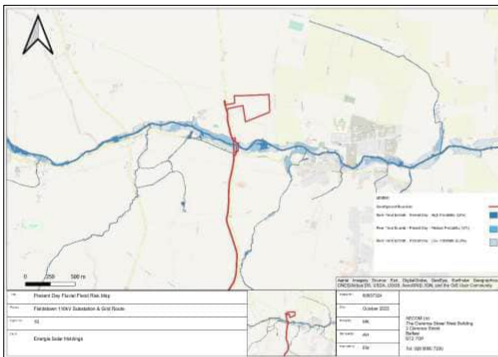
Figure 3-7 CFRAM Present Day Fluvial Flood Extents
